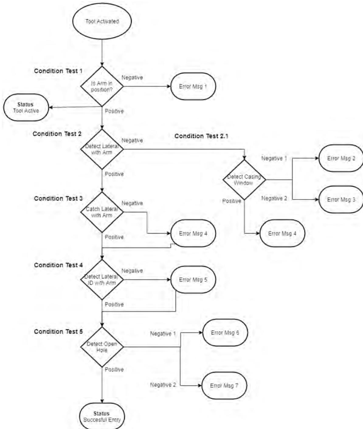
Figure 8—ALADIN algorithm flow chart
