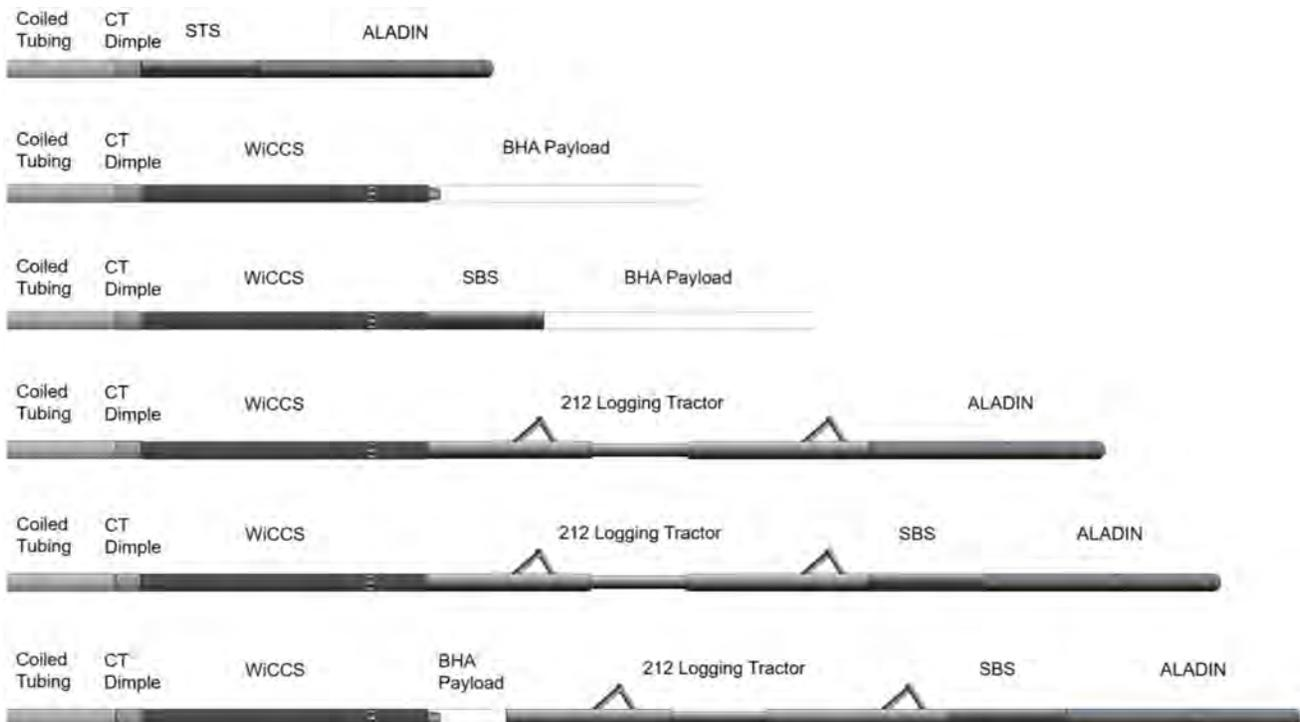
Figure 3—SASS configurations
